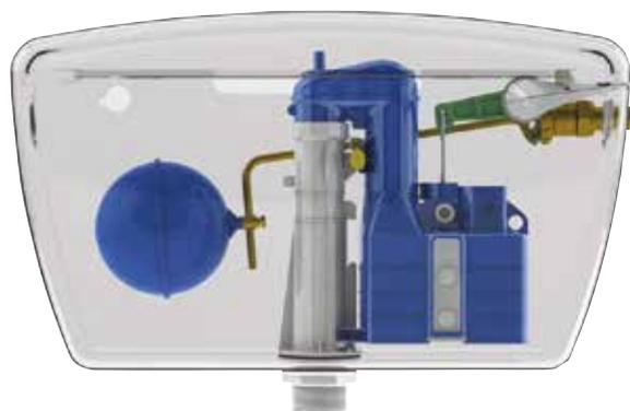
Water-saving flushing devices are now available to provide full and reduced flushing. Increases in new build and renovation has meant that single flush 9 litre cisterns are now commonly being replaced by dual-flush 6/4L, 5/3L and even 4/2.6L cisterns. They give the user the option of choosing a full flush for solids or a water-saving reduced flush for urine.
